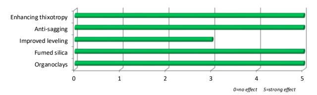
UNIQ®SPERSE P-405 is a liquid rheology additive for plastic applications such as vinyl ester and epoxy resins, unsaturated polyester resins, and gel coats. It can reinforce the rheological effectiveness of fumed silica and organophilic phyllosilicates (organoclays). By adding the additive, incorporation of the fumed silica is made easier, separation is prevented, and the thixotropic behavior increased or stabilized.
